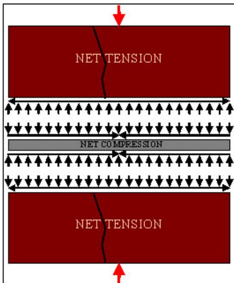
**Figure 19:** Free body diagram of compression induced tensile failure.
