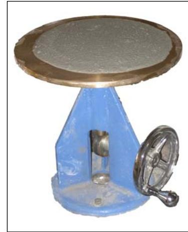
**Figure 7:** Mortar flow table after being dropped 25 times.
