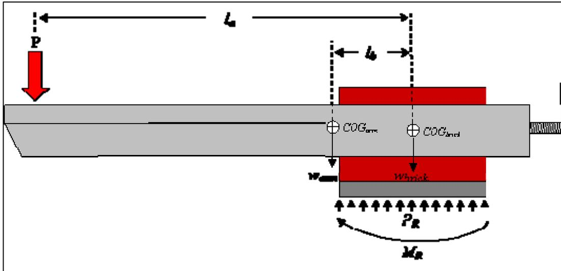
**Figure 18:** Free body diagram of bond wrench test specimen.
