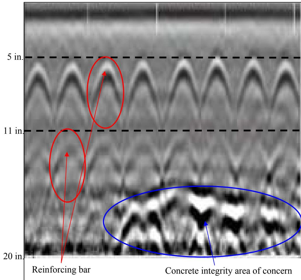
**Figure 23:** Characteristic radar return (Geophysical Survey Systems, Inc. 2006)
