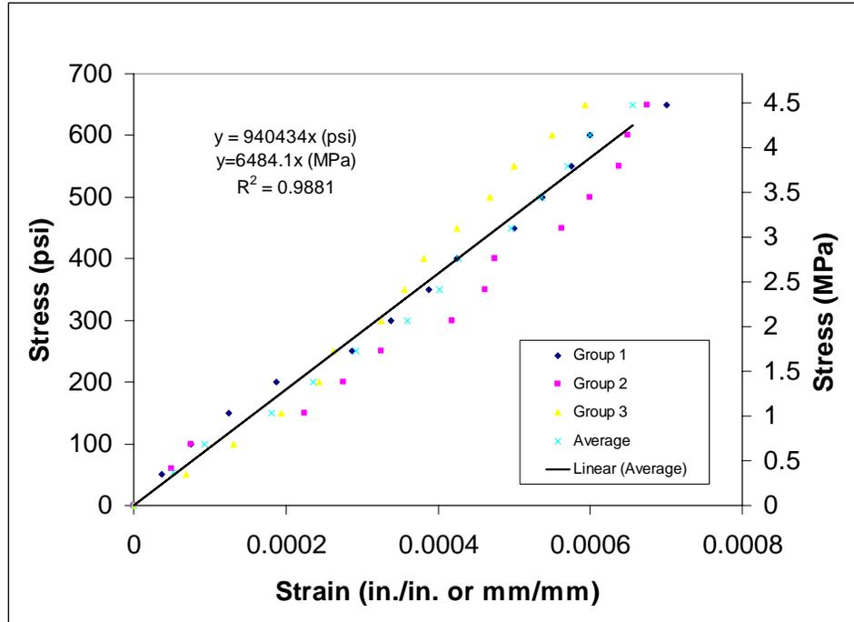
**Figure 33:** Sample modulus of elasticity test gage readings
