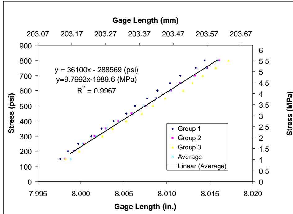
Figure 32: Sample in-situ stress gage measurements.
