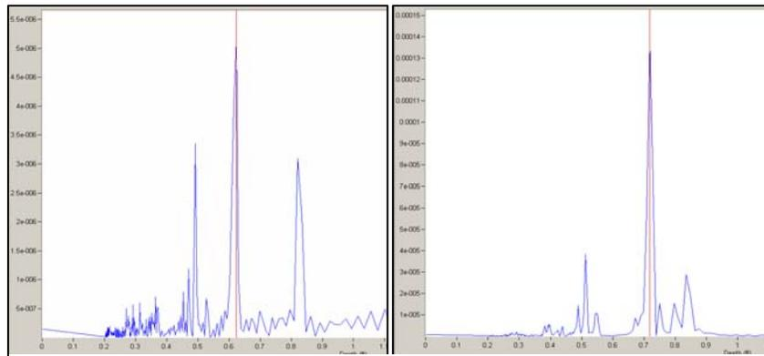
**Figure 28:** Impact-echo returns for sound cross section (left) and one with multiple simulated voids (right) notice the shift in return depths and magnitudes.
