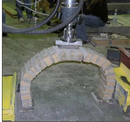
**Figure 21:** Masonry arch exhibiting failure during testing.
