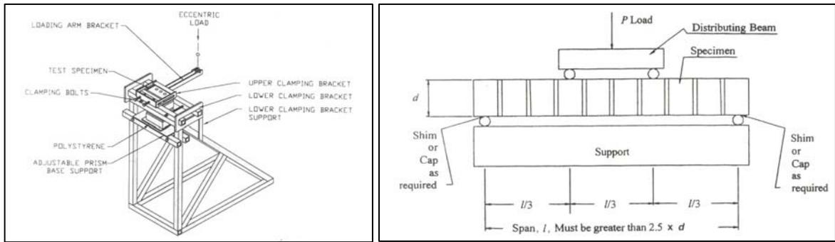
**Figure 14:** ASTM C 1072 test setup **Figure 15:** ASTM E 518 test setup (ASTM) (ASTM)
