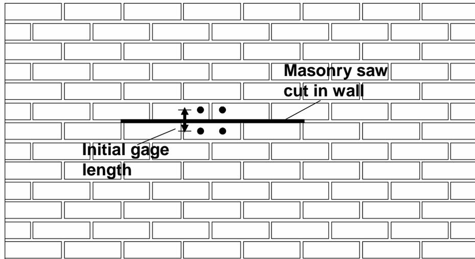
**Figure 29:** In-situ stress flat jack test setup.
