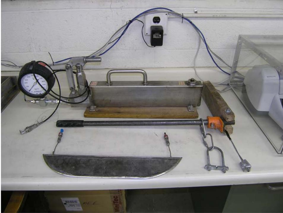
**Figure 31:** Flat jack test equipment: Pump (back), flat jack (front), and flat jack remover (middle and right).
