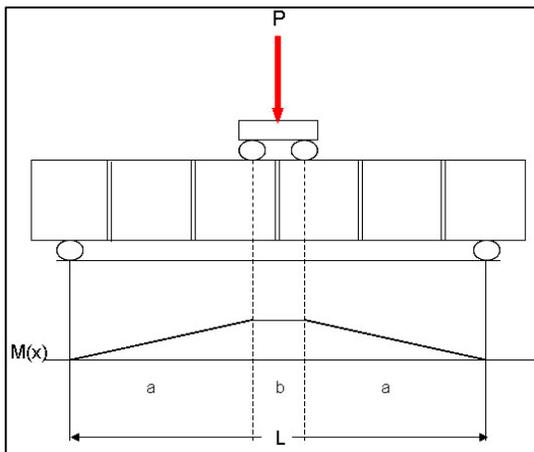
**Figure 16:** University of Wyoming's modulus of rupture bond strength testing (similar to ASTM E 518) test setup.
