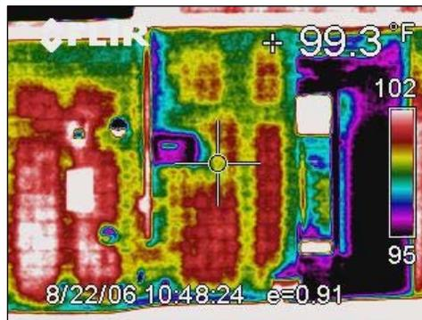
**Figure 35:** Infrared imaging of grout (cool) location in CMU wall.
