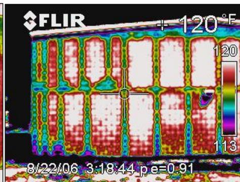
**Figure 36:** infrared imaging of grout (cool) location in CMU wall.
