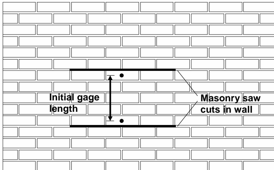
**Figure 30:** Modulus of elasticity flat jack test setup.
