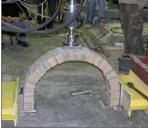
**Figure 22:** Masonry arch in test frame.
