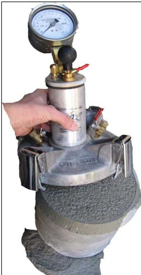
**Figure 8:** Mortar air entrainment measure by pressure method.
