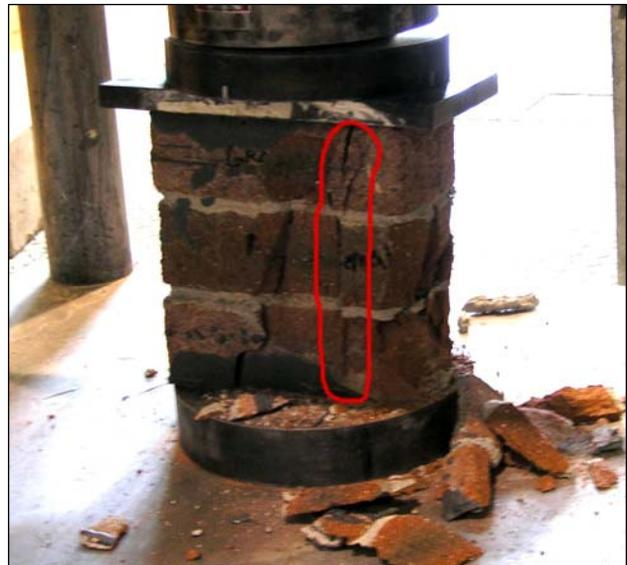
**Figure 20:** Compression failure of masonry prism due to induced tension.
