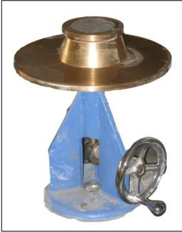
**Figure 5:** Mortar flow table with mortar mold in place.
