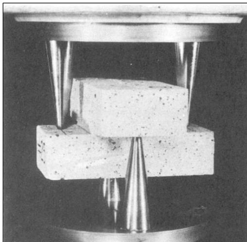
**Figure 12:** ASTM C 321’s crossed brick specimen in special loading apparatus.
