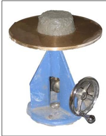
**Figure 6:** Mortar flow table with mortar mold removed.
