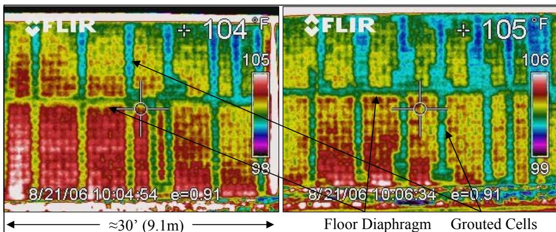
**Figure 24:** Characteristic infrared images of reinforced CMU wall, notice discontinuities in vertical grouting/reinforcing shown as the cooler regions.
