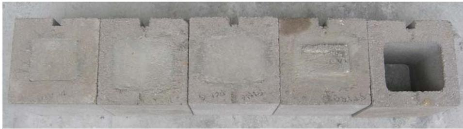
**Figure 27:** Impact-echo specimens from left to right: solid, one small void, many small voids, one large void, and empty
