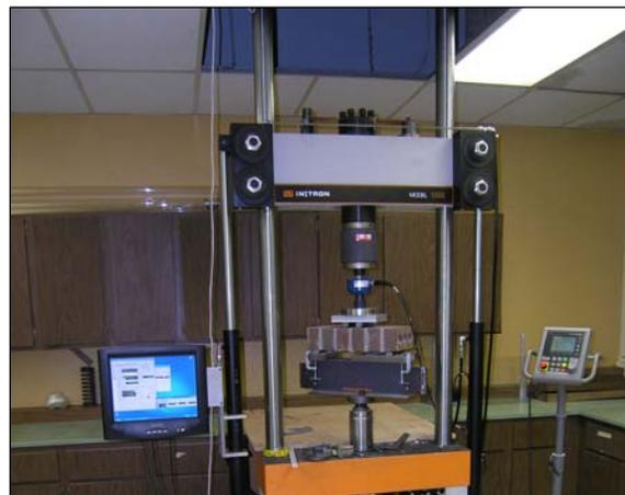
**Figure 17:** Modulus of rupture test equipment with specimen ready for testing.
