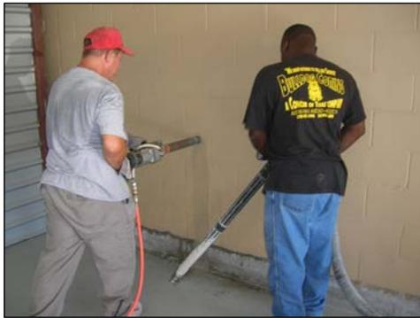
**Figure 39:** Drilling core samples for visual inspection and strength testing.
