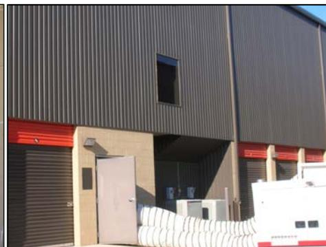
**Figure 38:** Cooling system utilized in infrared imaging of interior walls.
