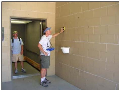
**Figure 37:** Locating steel reinforcement in CMU masonry wall with a cover meter.
