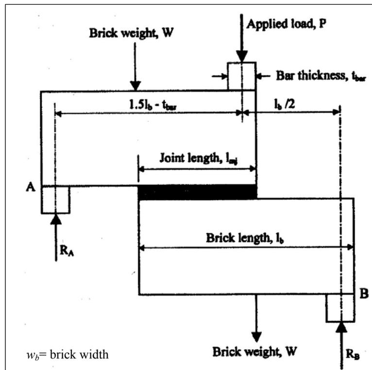
**Figure 13:** Khalaf's proposed Z brick orientation for bond strength testing. (Khalaf 2005)
