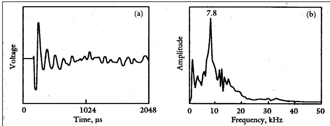
**Figure 26:** Complex return voltage (left) transformed to frequency domain (right) (Sansalone and Streett 1997).
