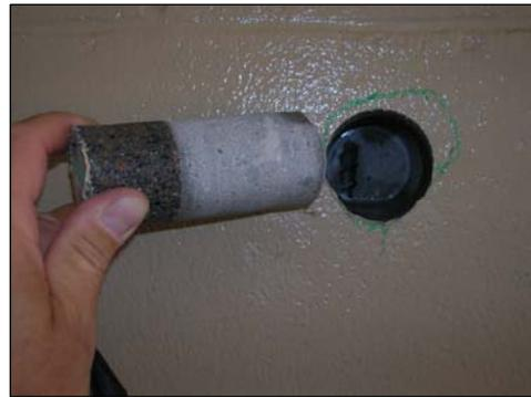
**Figure 40:** Characteristic core sample.
