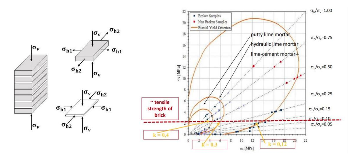
When unit is stiffer than the mortar
