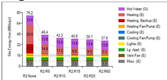
Duluth – Variation in wall insulation has an impact initially but tails off quite quickly. R 10 insulation gives close to maximum impact, beyond this there is little impact.
