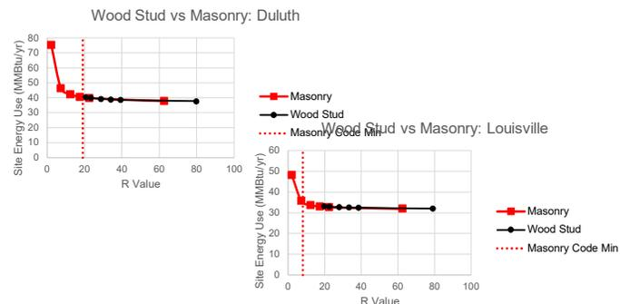
The prescriptive Code limits can be used to set insulation limits in passive house design. Note the Duluth prototype does not quite meet the 4.75 limit but gets close and does meet the climate limited
