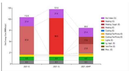
Heating Systems has significant impact in cold climates Duluth Minnesota
