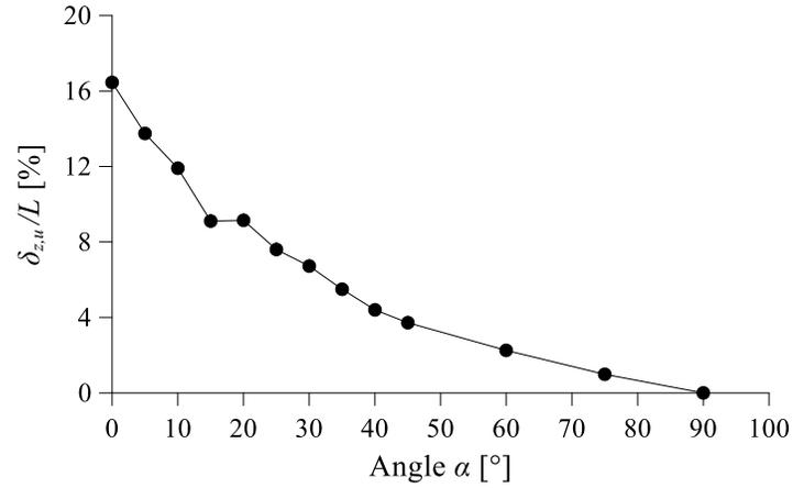
Vertical collapse displacement vs.  $\alpha$
