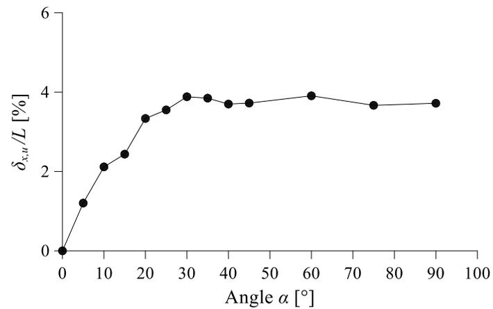
Horizontal collapse displacement vs.  $\alpha$
