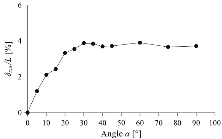
Horizontal collapse displacement vs.  $\alpha$
