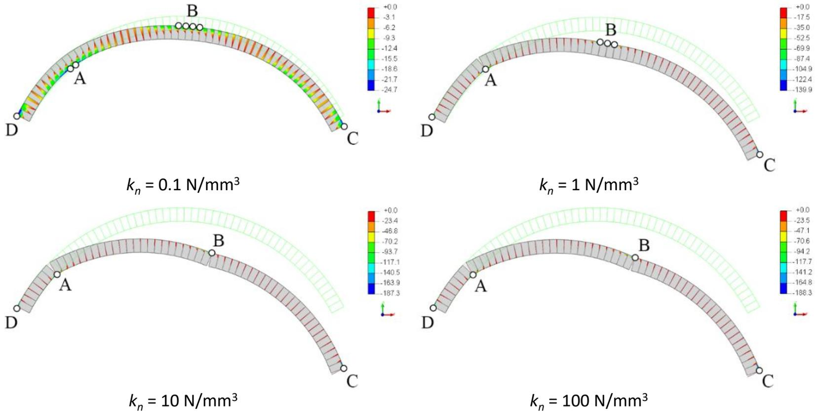
Collapse mechanism vs  $k_n$
