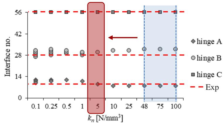
Hinge position at collapse vs  $k_n$
