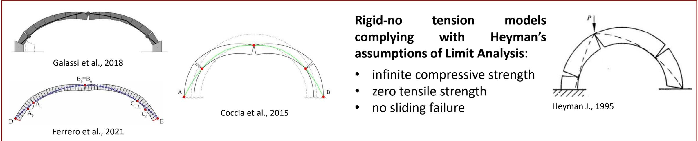
The figure contains four diagrams of masonry arches. The top-left diagram shows a grey arch on two supports. The bottom-left diagram shows a blue arch with points labeled  $D$ ,  $A_0$ ,  $A_u$ ,  $B_0=B_u$ ,  $C_u$ ,  $C_0$ , and  $E$ . The middle diagram shows a green arch with points  $A$  and  $B$ . The right diagram shows a black arch with a load  $P$  and a dashed line indicating a failure mechanism.
