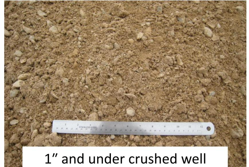
1" and under crushed well graded gravel
