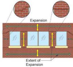
Figure 4.; BIA Tech Note 18A Accommodating Expansion of Brickwork
